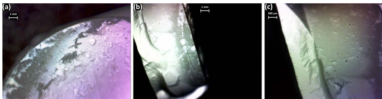
Figure 4. Optical micrographs of PMO exposed to HCl (15%) at 50°C and 41.4 MPa for 24 h in normal light: (a) 50× magnification, (b) 50× magnification, and (c) 150× magnification. [Color figure can be viewed in the online issue, which is available at wileyonlinelibrary.com .]
